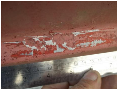
Spray rail damage
