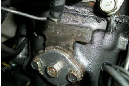
Fig 11 Peeled paint around head gasket
