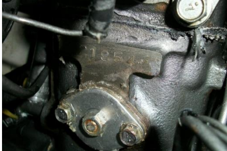
Fig 11 Peeled paint around head gasket
