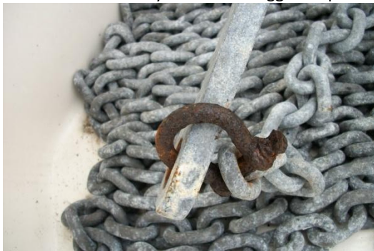
Fig 8 Corroded anchor shackle
