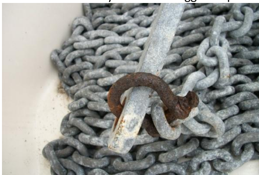
Fig 8 Corroded anchor shackle
