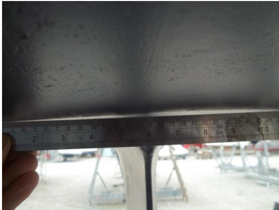
Hogging aft of the keel
