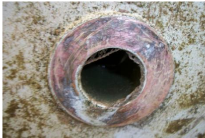
Fig 2 Dezincification around skin fitting
