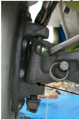
Fig 21 Gooseneck wearing at base. Fit bush
