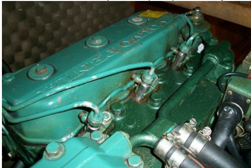
Fig 23 replaced injectors, painted head
