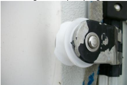
Fig 19 Genoa car broken
