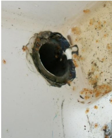
Fig 10 Cockpit drain gel coat breakdown.
