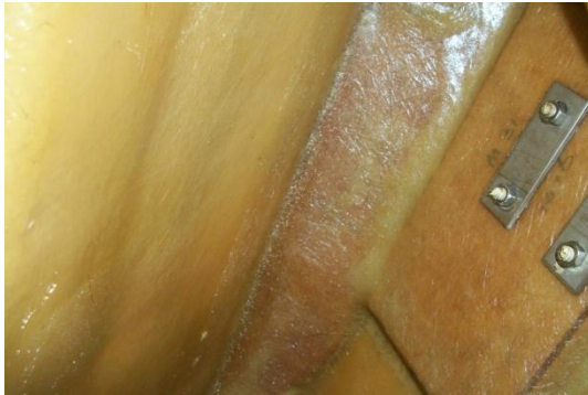
Fig 5 Deck moulding showing plywood strengthening and plates under fittings
