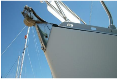
Fig 18 stem head bolt missing.
