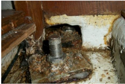
Fig 2, 3, 4 Surface corrosion on keel stud plates
