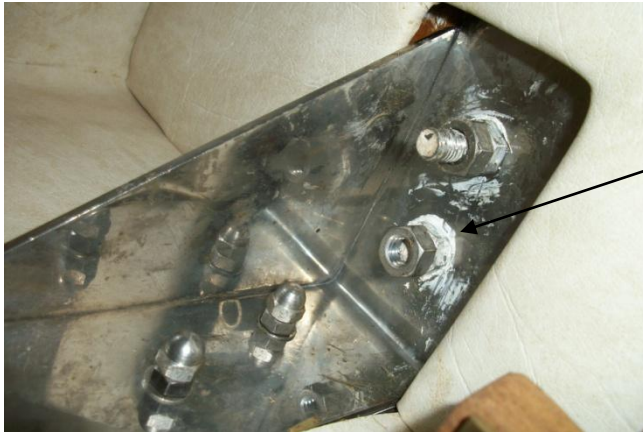
Fig 10 Note lock nut is not securely on thread.
