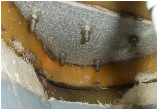
Underside stemhead and forestay fixing Underside starboard aft backstay fixing
